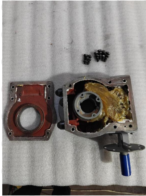
Photo 5:After waterproof test
