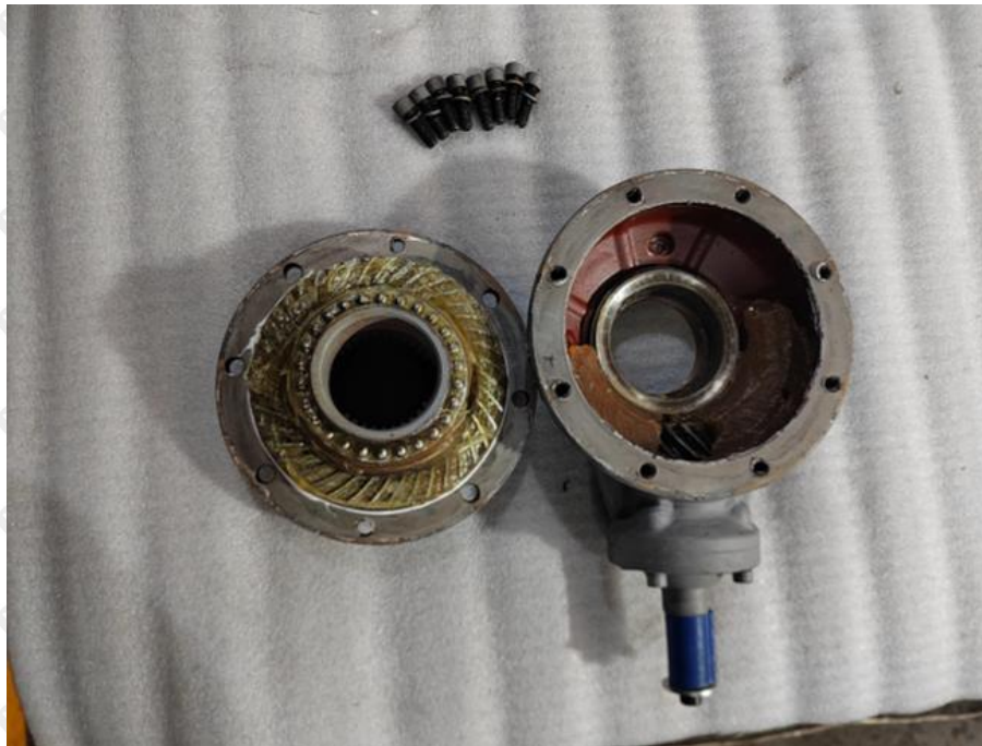
Photo 4:After waterproofing test
